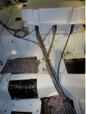
• Pass-through holes in sheet metal should have edges eased and there should be either a grommet in the pass-through hole or an abrasion resistant loom, wrap, sleeve, or tube surrounding cables and wires that pass through the hole.
