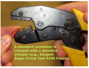
Use the correct die for the crimp connector (e.g., the red die should be used for the red crimp terminal, the blue die for the blue crimp terminal, etc.).
