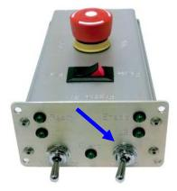
2. Disconnect power from the Ground Control Station's (GCS) GPS unit. This can be done at any point along the power cable (e.g., battery, wall connection, or power adapter).
