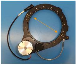
b. From the panhead screw side of the steering ring sub-assembly, remove the 2 panhead screws and lock washers along the seam opposite the hinge seam and closest to the motor.
