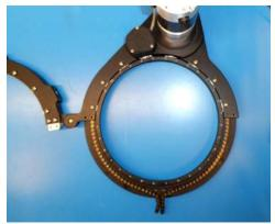
f. While maintaining the position of the motored half, loosely close the outer ring around the chained inner ring.
