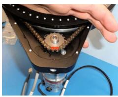
m. Place the steering ring sub-assembly on the workbench with the motor facing up.
