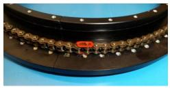
s. Use the ring pliers to squeeze the closed end of the chain hinge clip toward the protruding prongs until the chain hinge clip is firmly seated on top of the infinity chain hinge and under the protruding prongs' lips.
