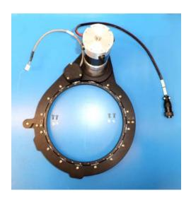
Replace all four panhead screws and lock washers removed in steps 1.a and 1.b.
