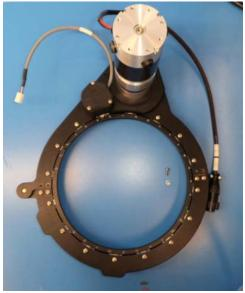
o. Open the outer ring with the non-motored half to the left.
