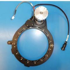
g. On the backside of the steering ring, replace the panhead screw and lockwasher removed in step 3.a.
