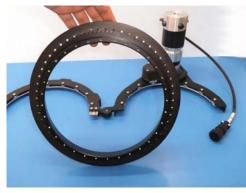
d. Set the center point of the steering ring chain at the top-rear of the internal ring, so that approximately equal lengths hang from the area adjacent to each bolt strip.
