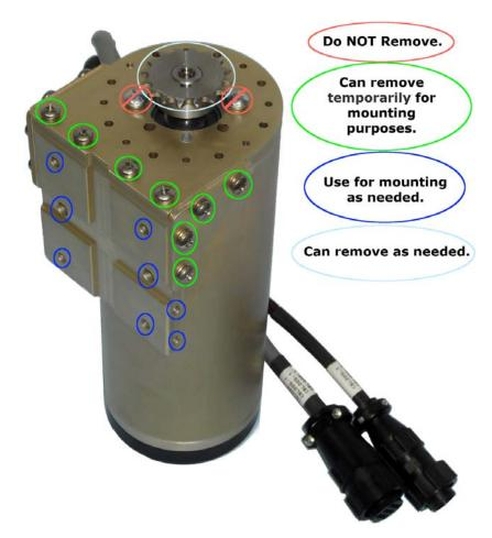
Company Confidential © 2013, Kairos Autonomi® Scalable Autonomy™ Pronto4 Steering Motor Module (No Steering Ring) Installation and Usage Notes v.01.00.01 Page 2 of 2 2014-06-03 / 16:48 Pronto4 Steering Motor Module (No Steering Ring) 01\_00\_00\_01.doc
