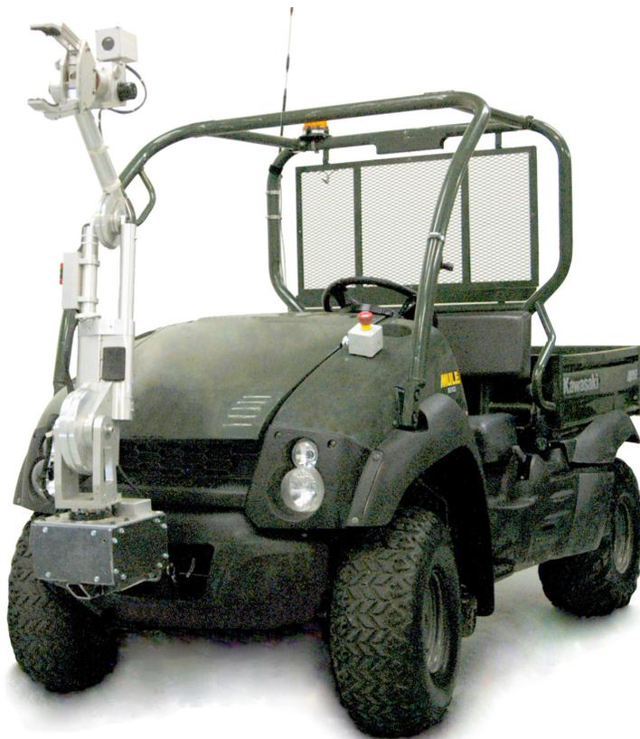
*A Kawasaki Mule retrofitted with the Pronto4™ Strap-on Autonomy System and a retrofit manipulator arm.*
