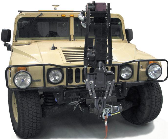
*A Pronto4 retrofitted HMMWV with a retrofit manipulator arm attached to the front. The arm can also be attached to the back of the vehicle.*
