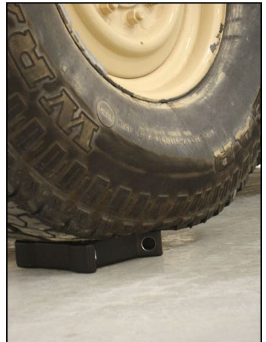
The Safety Direct enclosure can withstand being run over by large vehicles. Pictured above, the enclosure is underneath a commercial Hummer (6500 lbs.).
