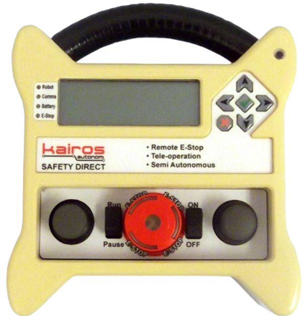
The Safety Direct Wireless E-stop and Handheld Controller
