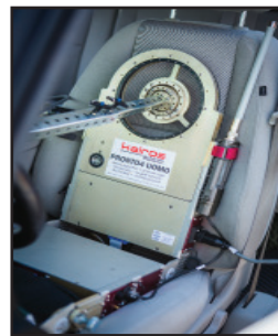
The Pronto4 Uomo steering mechanism (left) utilizes a high angle gimble to control the steering wheel. The Pronto4 Uomo's feet (right) control the brake and throttle pedals.
