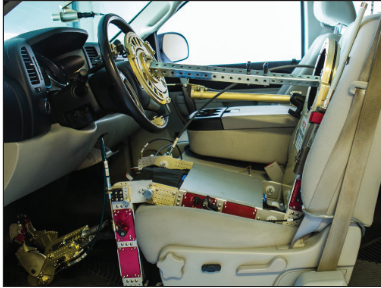
The Pronto4 Uomo controls the vehicle from the driver's seat. In about 10 minutes, the Pronto4 Uomo can be installed in a vehicle and control, steering, brake, throttle and transmission.
