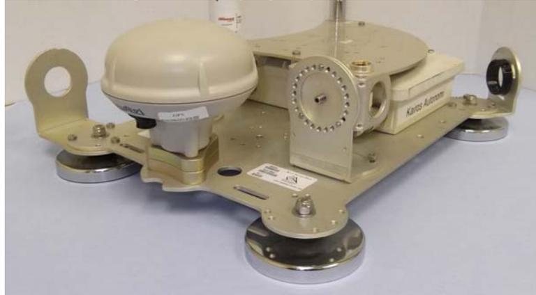
2. Use a #2 Phillips driver to remove the attached GPS hardware (i.e., screws and lockwashers).
