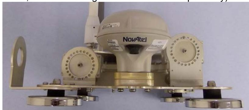
6. Run the GPS cable's long pigtail (CBL-045, end marked "to GPS") down through one of the two large round holes (identified in step 1) then up the outside of Roof Rack and into the GPS's cable connector. Connect the GPS cable. The cable is run this way to provide tension relief and ensure the connector is connected squarely to the GPS.
