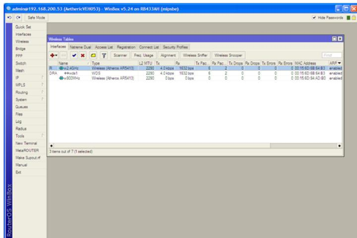
3. At the top of the “Interface <frequency>” window, click the “Status” tab. On the Status tab, locate the “Noise Floor” entry. Noise floor should be between -90 and -100dBm. A value between -80 and -90 is marginal. Anything more than -80 is challenging. Also note the “Frequency” value for the next step.
