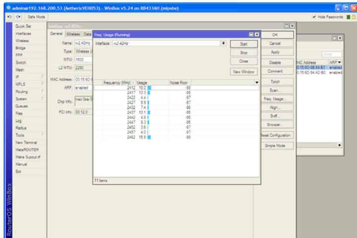
7. In the upper-right corner of the “Freq. Usage” window, click the “Stop” button to stop scanning. Failure to stop scanning will prevent scanning by other tools. Click the “Close” button to close the “Freq. Usage” window.
