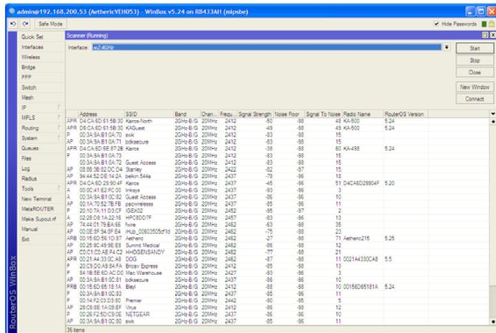
5. In the upper-right corner of the “Scanner” window, click the “Stop” button to stop scanning. Failure to stop scanning will prevent scanning by other tools, including the frequency usage scanner to be used in the next step. Click the “Close” button to close the “Scanner” window.
