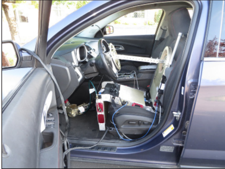
The Pronto4 Uomo controls the vehicle from the driver's seat. In about 10 minutes, the Pronto4 Uomo can be installed in a vehicle and control the steering, brake, throttle and transmission.
