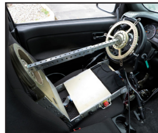
The Pronto4 Uomo steering mechanism (left) utilizes a high angle gimble to control the steering wheel. The Pronto4 Uomo's feet (right) control the brake and throttle pedals.
