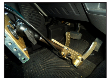
The Pronto4 Uomo steering mechanism (left) utilizes a high angle gimble to control the steering wheel. The Pronto4 Uomo's feet (right) control the brake and throttle pedals.
