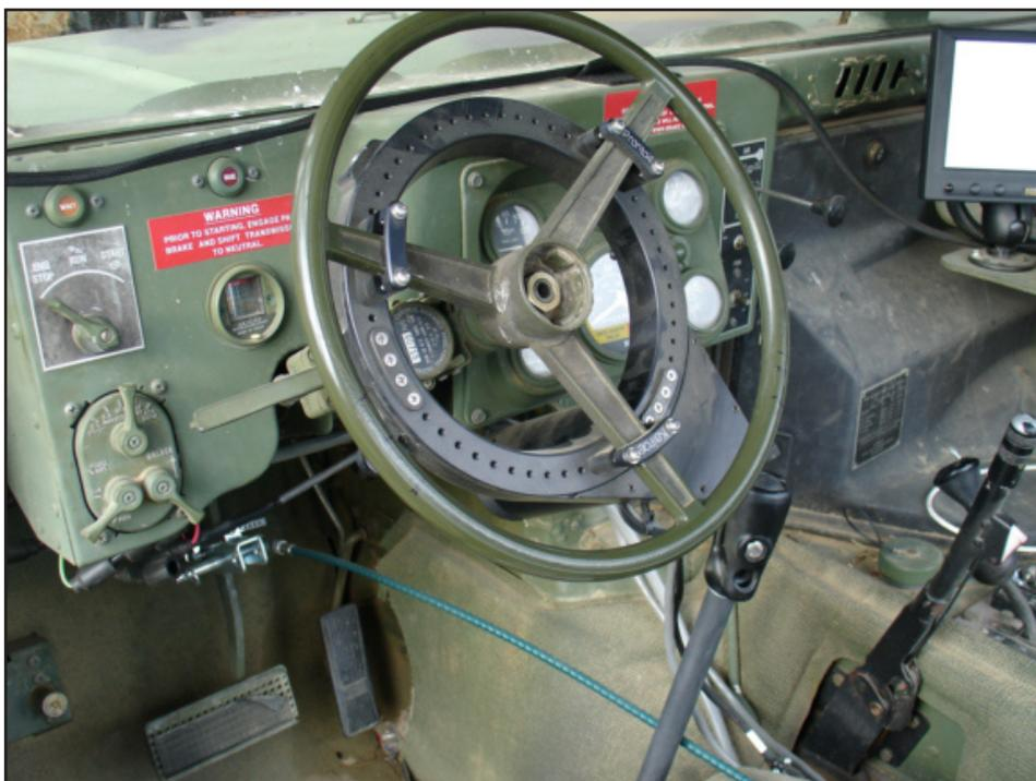
A Pronto4™ Strap-on Autonomy System Series 2 installed on a military HMMWV.
