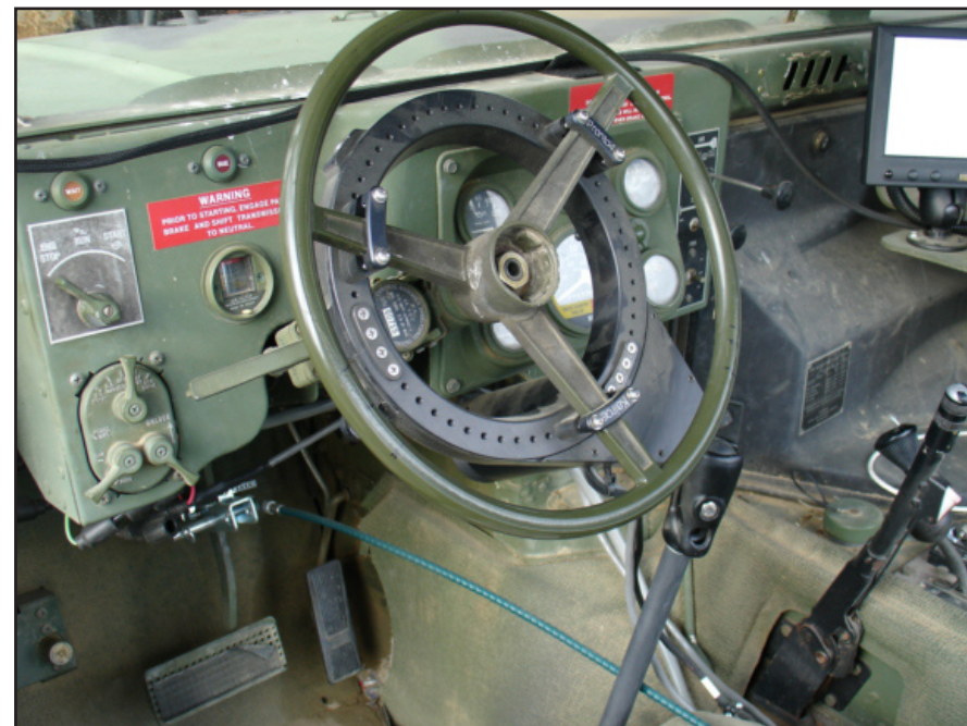
A Pronto4™ system installed in a military HMMWV.
